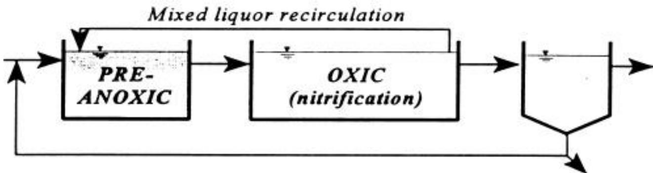
The anoxic basin is mixed, but not aerated. Mixers can be floating mechanical type or submersible motors fitted with propeller type mixers.
